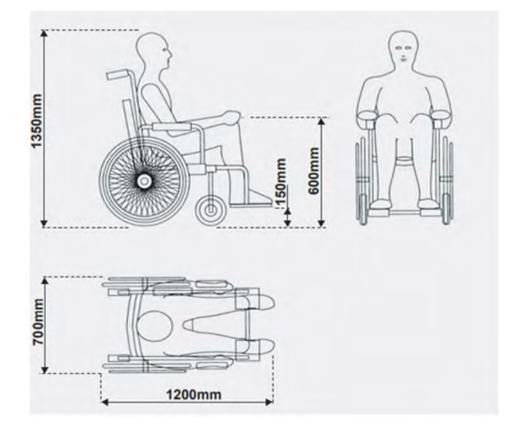
848. The reference wheelchair has: a total length of 1200mm including extra-long footplates total width of 700mm sitting height (from ground to top of head) of 1350mm. The reference wheelchair is bigger than most wheelchairs to ensure that enough room is provided for most wheelchair users.
